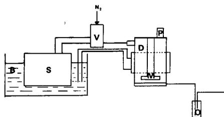
Fig. 1. Diagrammatic representation of the experimental apparatus. D is the ultrafiltration cell fitted with a stirrer M. A reservoir S containing solvent is kept in a constant temperature bath B, water from which also circulates around D. The switch V allows pressure to be applied to S, D or both. Immediately below the stirrer M is a membrane supported on a sintered disc. The emerging solution is passed through a flow cell O.
