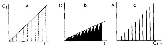
Fig. 3. Schematic depiction of the simulated dissolution experiment using FISDD system. a, linear change of drug concentration ( $C_t$ ) in the dissolution medium according to Eqn. 1; b, change of drug concentration  $C_i$  in the receiving solution of successive dialysis runs according to Eqn. 3. The concentrations  $C_{i,t}$  correspond to the maxima of  $C_i$  peaks; c, recorded FIA absorbance peaks at successive injections according to Eqn. 5.
