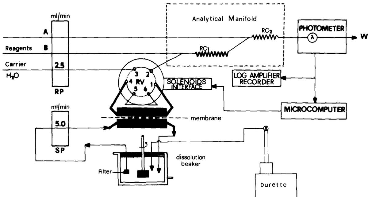
Fig. 1. Schematic diagram of flow injection serial dynamic dialysis (FISDD) system for dissolution studies in milk. RP, reagent pump; SP, sample pump; RC1, RC2, reaction coils; W, waste; RV, rotary valve.
