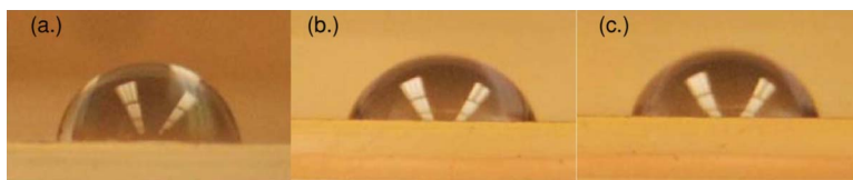
Fig. 4. Sample contact angle images for (a) deionized water, (b) deionized water with added aspartame, and (c) deionized water with added potassium benzoate. Note that the contact angle for the aspartame and potassium benzoate solutions is less than the contact angle for pure water, indicating a decrease in the surface tension.
