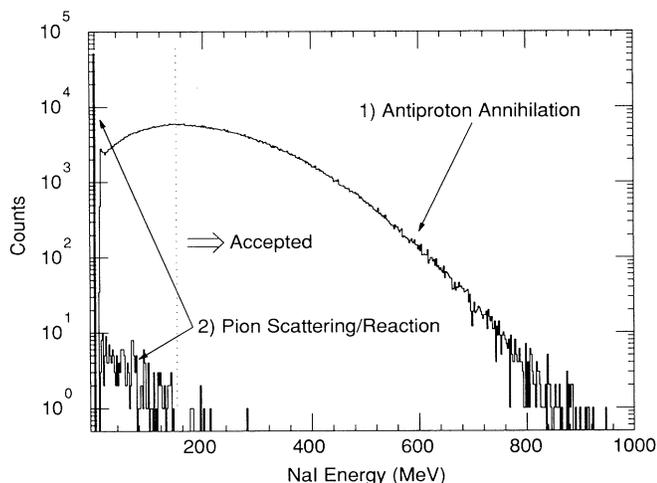
FIG. 1. Energy-sum spectra of the NaI counters corresponding to (1)  $\bar{p}$  annihilation events and (2) pion scattering and reaction events.
