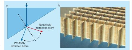
Figure 1 Negative refraction. a, Light incident on a normal material refracts at a positive angle (blue), but in a negative-index material the refraction angle is negative (red). Negative refraction occurs only in specially engineered materials. b, This arrangement of fibreglass sheets (1 cm high) in which is embedded an array of copper loops and wires was the first 'material' for which negative refraction was seen<sup>2</sup>.
