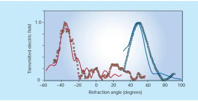
Figure 2 Negative refraction confirmed. These data from Parazzoli *et al.*<sup>3</sup> compare refraction in their negative-index material (red points) with the response of a normal, positive-index material, Teflon (blue points). Moreover, the experimental data are in fair agreement with simulations (solid lines).
