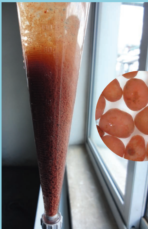
Going red. With this cone, engineers gauge the density of the clumps of red anammox bacteria ( inset ), a new way to denitrify wastewater.
