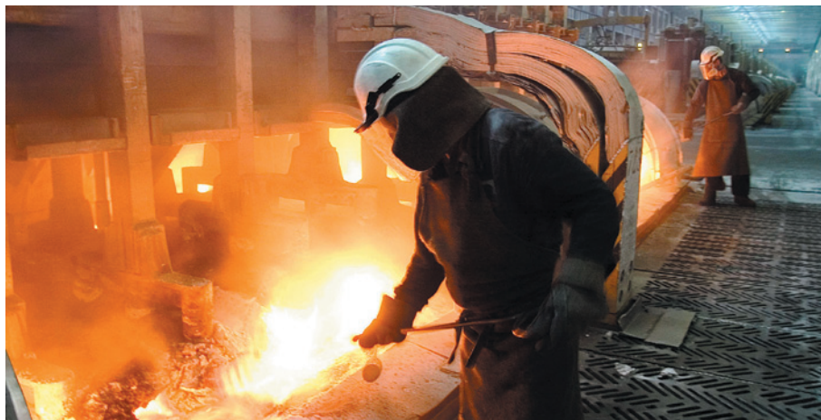
Figure 1 | Metal extraction by electrolysis. The interior of an aluminium smelter demonstrates the harsh conditions that must be withstood by the components of electrolytic cells. Allanore et al. 2 report materials that could be used as anodes in the electrolytic production of iron.
