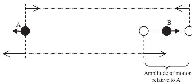
Figure 3. The bond-stretching effect. When the mean distance between atoms A and B is held constant, vibrations along the bond direction produce a net repulsive force: the pair potential is asymmetric (figure 1), and so the attraction when the atoms are further apart is smaller than the corresponding repulsion when they are closer together. \rightarrow , instantaneous force; \Rightarrow , time-averaged force.
