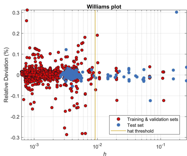
FIG. 5. Williams plot of the SVR correlation for the density data of the (water + KCl) system. The hat values are calculated using Eq. (12) for the training and validation sets and for the test set.
