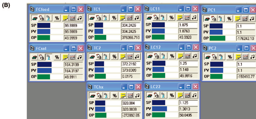
Figure 7. (A) Control structure CS1; (B) controller faceplates.
