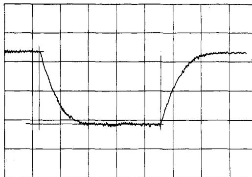
Figure 1. Electron current vs. time observed in pure neopentane at  $E = 198 \text{ V/cm}$ ; vertical scale, 1 major division =  $2 \times 10^{-8} \text{ A}$ ; horizontal scale, 1 major division =  $50 \mu\text{sec}$ .  $T = 23^\circ$ .
