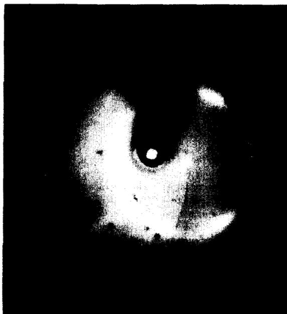
FIG. 1. LEED pattern of one-dimensionally ordered structure of monolayers of the *n*-paraffins on Pt(111). (42 V incident beam).
