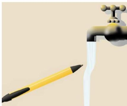
Figure 1 Polarized water. In a simple experiment, a stream of tap water is deviated by the static electricity of a plastic pen (which has previously been charged by rubbing on wool) because the water molecules are partially aligned in the electric field.
