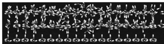
FIG. 8. A three bilayer PUCKERED model, top and side view, after the 178 ps trajectory, before recooling. The initial structure was ferroelectric.
