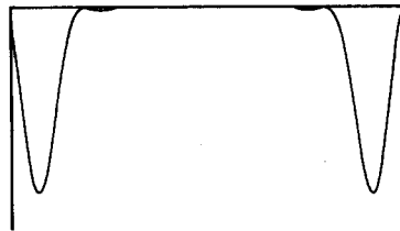
Fig. 16. Infinite square well wave packet at one-quarter period. Although each lobe is smaller than the original, they appear the same size because of scaling.
