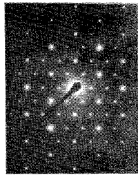
FIG. 2: The unit cell of reciprocal lattice constructed from various reciprocal lattice planes observed by electron diffraction.
