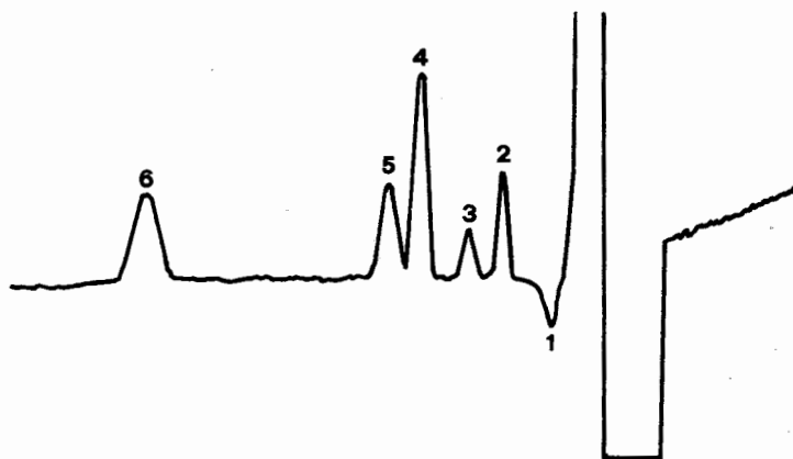
FIG. 3: Standard chromatogram of F - 1 ppm, Cl - 1 ppm, NO 2 - 1 ppm, Br - 5 ppm, NO 3 - 2 ppm and SO 4 2- 2 ppm using eluent KHP 4 mM and pH: 4.9
