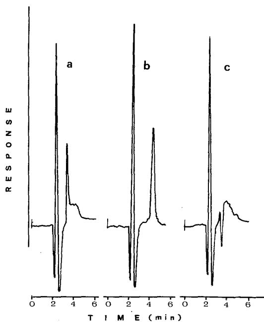
FIG. 1 Chromatograms of an aqueous solution of tetracycline extracted with ethylacetate (a) or dichloromethane (b) ; a chromatogram (c) of control water extracted with ethylacetate is presented. Mobile phase: \text{CH}_3\text{CN}-\text{H}_2\text{O} (20:80) with 0.01M \text{NaH}_2\text{PO}_4 , pH 2.6 with \text{HNO}_3 ; column: 2.6X250 mm HC-ODS-SIL-X-1 (10 \mu\text{m} ); column temperature: 30 ^\circ\text{C} ; flow rate: programmed (see text); detector: UV, \lambda = 361 \text{ nm} ; recorder sensitivity: 0.020 a.u./s.
