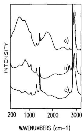
Figure 10. FT-Raman spectra in the 200–3200 \text{cm}^{-1} region (1.064 \mu source). (a) Sm-EMAA (5.4 mol % \text{Sm}^{3+} ), (b) Dy-EMAA (5.4 mol % \text{Dy}^{3+} ), (c) Er-EMAA (5.4 mol % \text{Er}^{3+} ). The absorbance scale and the display offset are arbitrary.
