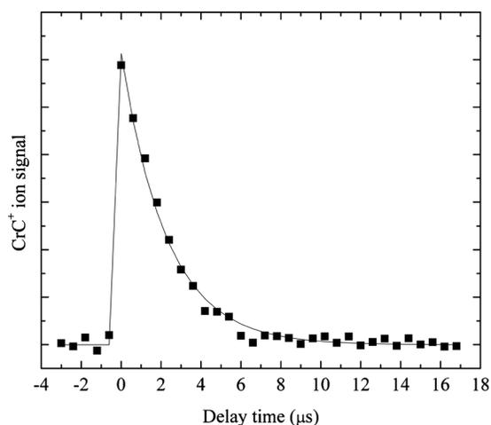
FIG. 2. Excited state decay measurements for the 11 871 cm<sup>-1</sup> band (data points) and fitted decay curve (solid line). Based on four independent measurements of this decay curve, the upper state lifetime is found to be  $2.06 \pm 0.17 \mu\text{s}$  ( $1\sigma$  error limit).
