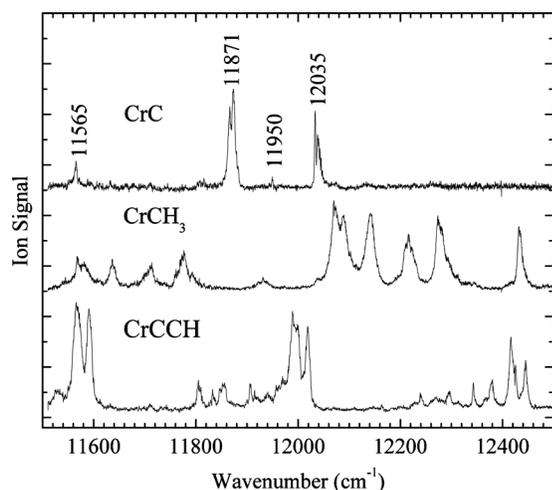
FIG. 1. Vibronically resolved spectra of jet-cooled CrC, CrCH<sub>3</sub>, and CrCCH produced by laser ablation of chromium metal in a supersonic expansion of 3% CH<sub>4</sub> in helium.
