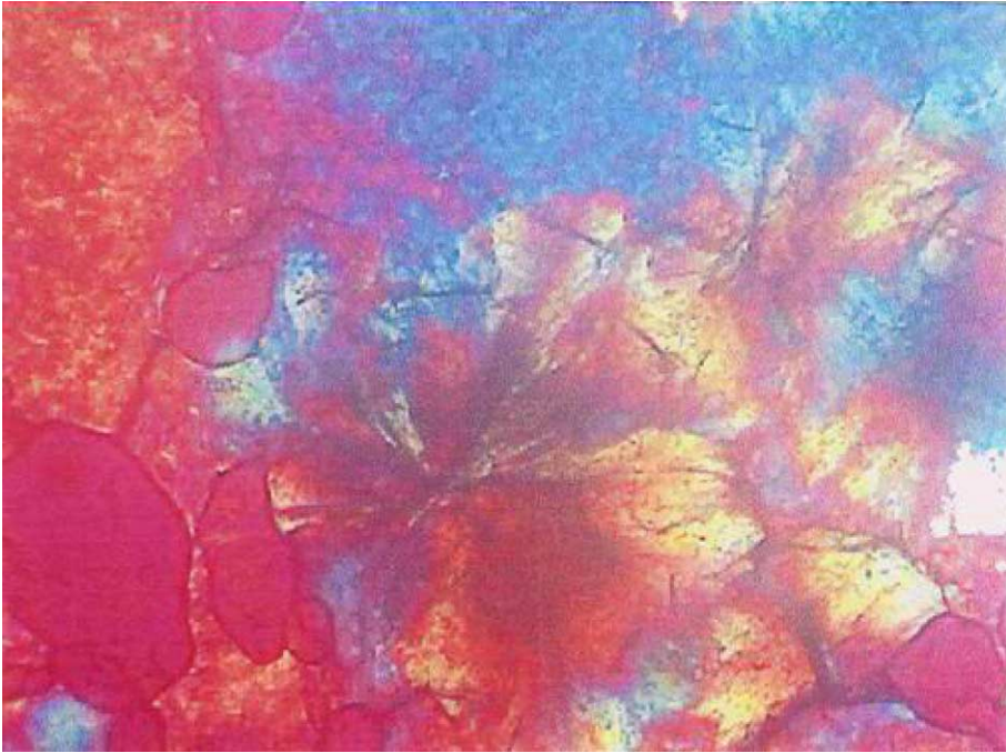
Fig. 4. Optical microscopy micrograph for sample 2-amino-hexadecanol at 60 °C.
