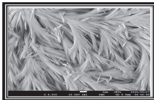
FIGURE 1. FESEM image of SrCO 3 superarchitecture
