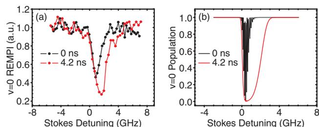
FIG. 4. SARP-induced population transfer (a) experimental REMPI signal and (b) theoretical fractional population in  $\nu = 0$ ,  $J = 0$  state for two different relative delays  $\tau_D = 0$ , and  $4.2 \text{ ns}$  between the 6 ns (intensity FWHM) pump and 4.5 ns Stokes laser pulses. The pulse energies are nearly the same as in Fig. 3.
