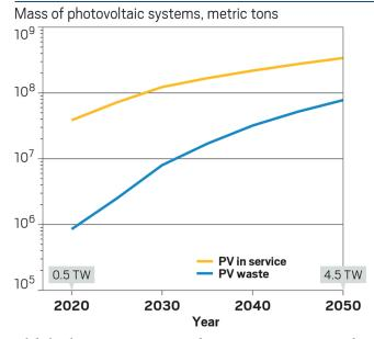
Global solar capacity is expected to grow to 4.5 terawatts by 2050, but this will create a growing burden of photovoltaic waste that could hit 80 million metric tons by the same year. Credit: Adapted from *Nat. Energy* **2020**, DOI: 10.1038/s41560-020-0645-2, with permission
