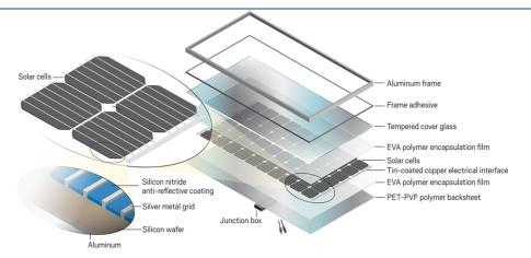
Solar photovoltaic modules are a complex sandwich of metals, semiconductors, polymers, and glass that is built for durability but difficult to disassemble. Credit: Adapted from *Nat. Energy* 2020, DOI: 10.1038/s41560-020-0645-2, with permission
