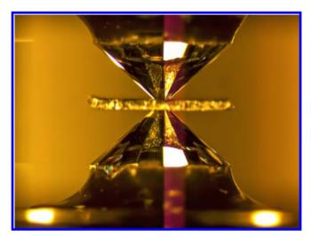
In a diamond anvil such as this one, two diamonds squeeze a cell filled with a material. At high pressures, certain materials could become superconductors. Credit: Steven D. Jacobsen.
