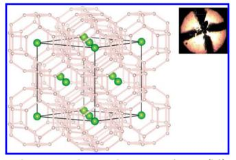
Hydrogen atoms dominate the structure of  $LaH_{10}$  (left). Lanthanum is green and hydrogen is white. A sample of superconducting  $LaH_{10}$ , seen through a diamond anvil, sits centered among four black electrodes in a 50  $\mu$ m wide cell (top right). Credit: Russell Hemley.
