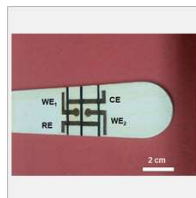
IMAGE: ELECTROCHEMICAL CELLS ETCHED BY A LASER ON A WOODEN TONGUE DEPRESSOR CAN MEASURE GLUCOSE AND NITRITE LEVELS IN SALIVA. (WE = WORKING ELECTRODE, CE = COMMON COUNTER ELECTRODE, RE = COMMON REFERENCE ELECTRODE) view more >
